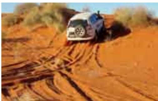
Higher pressures will be required when carrying heavy loads. Sudden or heavy movements of the steering can be dangerous and speed needs to be appropriately reduced depending on the depth of the sand. Sand can vary rapidly in patches. Sand can also build up a lot of heat in your tyres because you are running lower pressures for flotation, so you may need to rest your vehicle regularly. Sand creates the most constant resistance to tyres, gearboxes and motors out of all mediums and applications.
